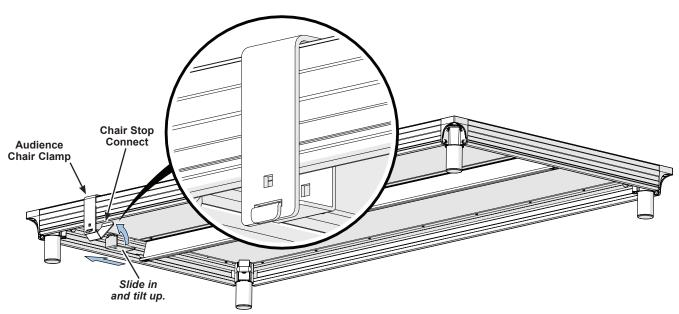
3. Secure together using a 3/8-16 x 3" carriage bolt and a 3/8-16 wing nut. Leave the connection loose enough to allow the location to be adjusted from side to side.
